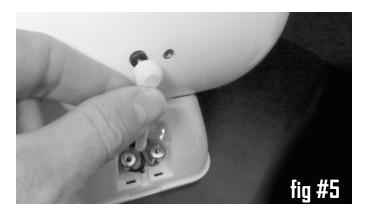
Now it very INPORTANT to attach the safety cable to the back of the speaker. See Figure #6 Even though the mount will safely hold the speaker the safety cable will prevent the speaker falling in an earthquake or something hitting it.
